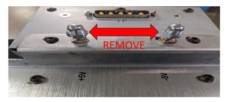
This cover is used to protect the potentiometers during shipping.
