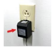
When **disconnecting** Patient Alarm Unit Box, remove the power adapter from the wall outlet <u>**BEFORE**</u> unplugging the power cable from the box.
